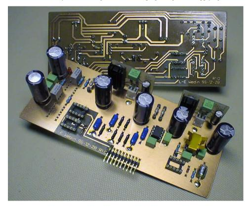
Figure 2 shows the prototype implementation of the 2-pole low-pass filter with differential input as is recommended by Crystal Semiconductors, notice the heat sink on AD811. Relays and input buffers have been removed from this pcb.
