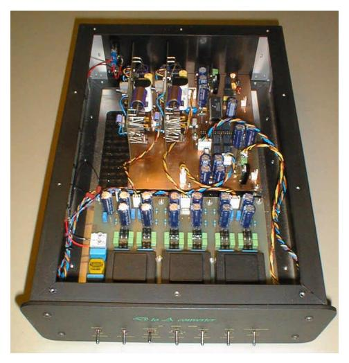
Figure 1 shows the interior of the Proto-DAC, sans the plug an play board containing the AD1890/91 sample rate converter, oscillators and dividers.
