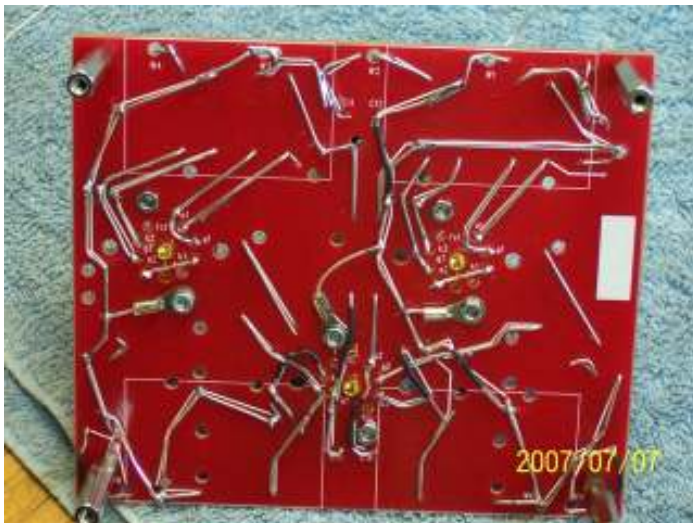
The underside of the board shows the 4 capacitors installed into position and soldered.
