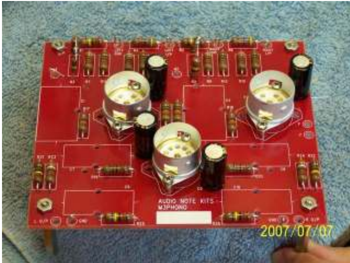
The top level view of the board with the capacitors installed.
