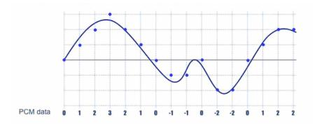
In the example above, the blue dots represent the sample points taken of this audio signal. The vertical lines represent the sampling frequency, or rate. This is defined in hertz, representing how many "readings' are taken each second. The horizontal lines represent the bit-depth, or resolution. The first thing you will notice is that the dots do not accurately represent the original signal. This is because the resolution in this example is quite low.
