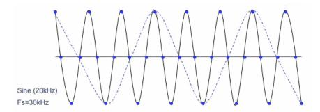
As we mentioned, the human hearing range tops out at about 20 kHz, and the Nyquist theorem shows that we need to sample at slightly faster than double that. This is how CDs ended up using 44.1 kHz as their sampling frequency. It is the lowest rate that assures accurate sampling through the entire hearing range.
