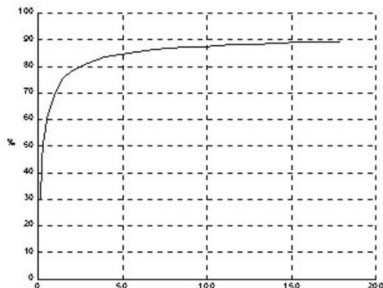
Figure 6: Efficiency vs. output power ( $4\Omega$ ).
