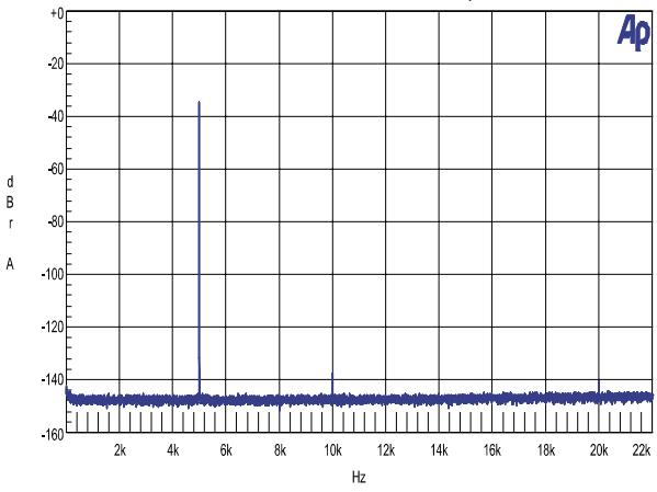
FFT Analysis.  $f = 5\text{kHz}$ .  $P_o = 100\text{mW}$   $4\Omega$  loading. THD = -101dB (0.0009%)
