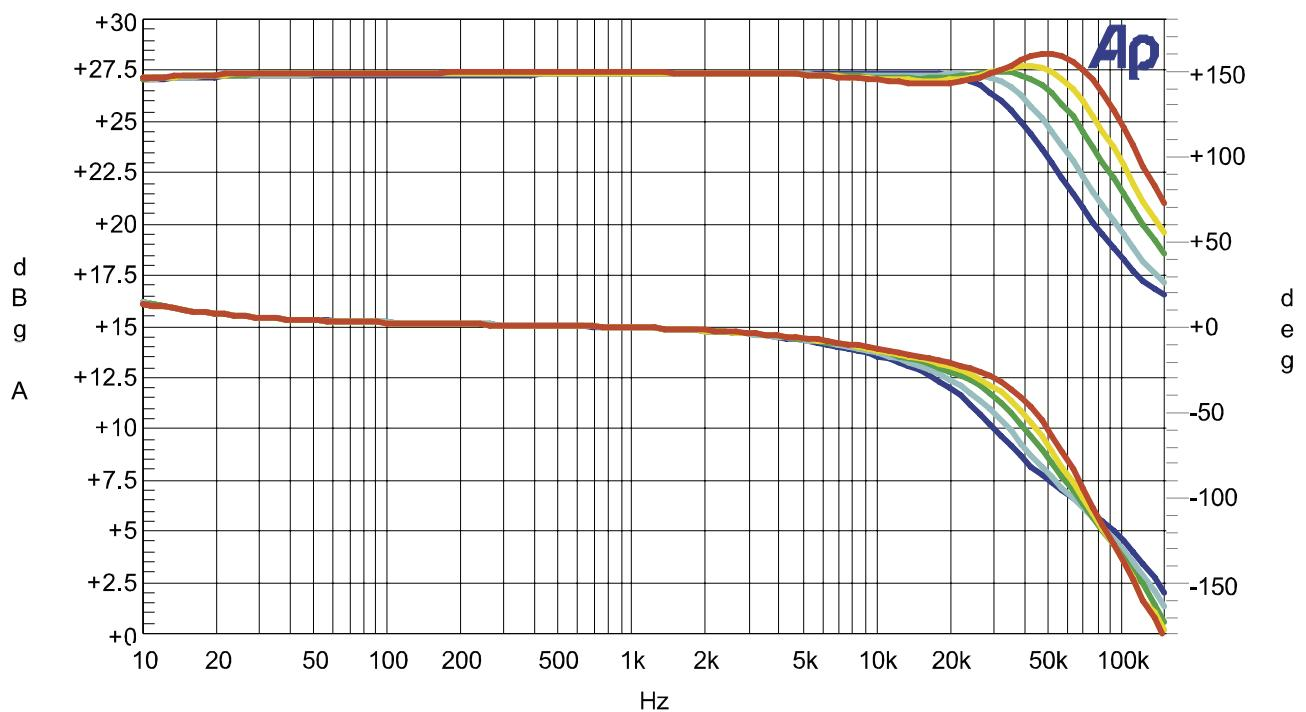
Figure 4: Frequency response in  $2.7\Omega$ ,  $4\Omega$ ,  $8\Omega$ ,  $16\Omega$  and open load. Top – amplitude. Bottom – phase.
