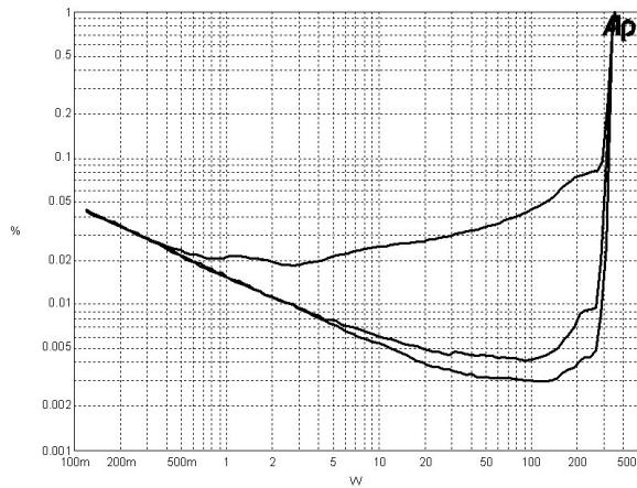
THD + N vs. output power at 100Hz, 1kHz and 7kHz<sup>4)</sup> (2.7Ω).
