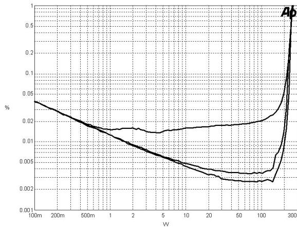
THD + N vs. output power at 100Hz, 1kHz and 7kHz<sup>4)</sup> (4Ω).
