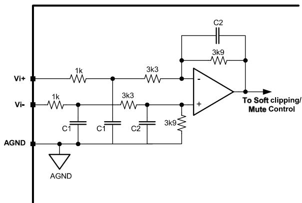
Figure 10: Balanced input buffer / anti-aliasing filter.
