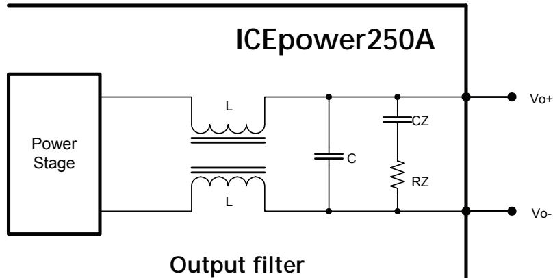
Figure 11: Output filter section with compensating Zobel network.
