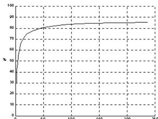
Figure 7: Efficiency vs. output power ( $2.7\Omega$ ).
