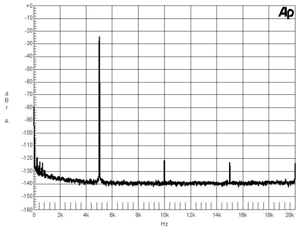
$f = 5\text{kHz}$ .  $P_o = 1\text{W}$ .  $4\Omega$  loading. THD = 0.002%.
